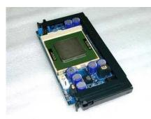
The PL-P3/SMP with installed processor.
